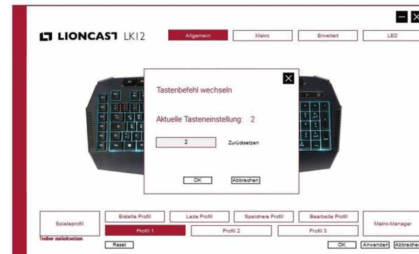
By clicking on the input field, a different function can be assigned to the selected key. Simply enter the new key in the input field and confirm with **[OK]**. By pressing **[Apply]** the setting will be transmitted to the keyboard. This may take a few seconds. The **[Cancel]** button discards the selected changes.
